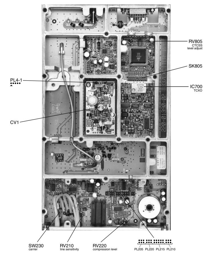
Figure 4.5 T837 Main Tuning & Adjustment Controls
